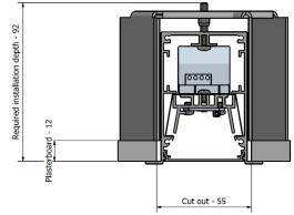
Please Note: This is for single 12.5mm plasterboard – if double plasterboard is being used to please contact us as we can offer a longer rod to fit the bracket.
